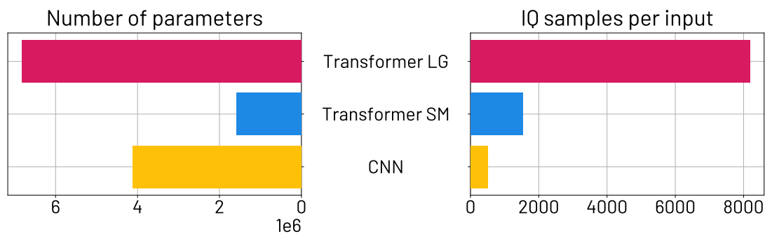
Figure 9: Comparison in model sizes both in terms of number of parameters of each architecture and number of IQ samples needed to do inference over the input.
